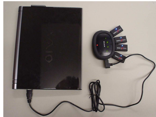
Figure 9: The Bluetooth content delivery server: We used a Sony Vaio X505 laptop equipped with four Bluetooth radios to serve content to all passing Bluetooth devices. One Bluetooth radio was responsible for discovering new devices, while the remaining three used BlueMonarch to serve content to all discovered devices.
